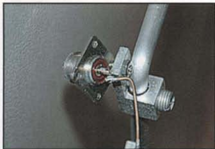
My 2-meter KU4AB square Halo omni antenna. The wire going to the center pin of the coaxial connector separated. This required a bit of cleanup and a resolder job using quality solder and some flux. (K7SZ photo)
