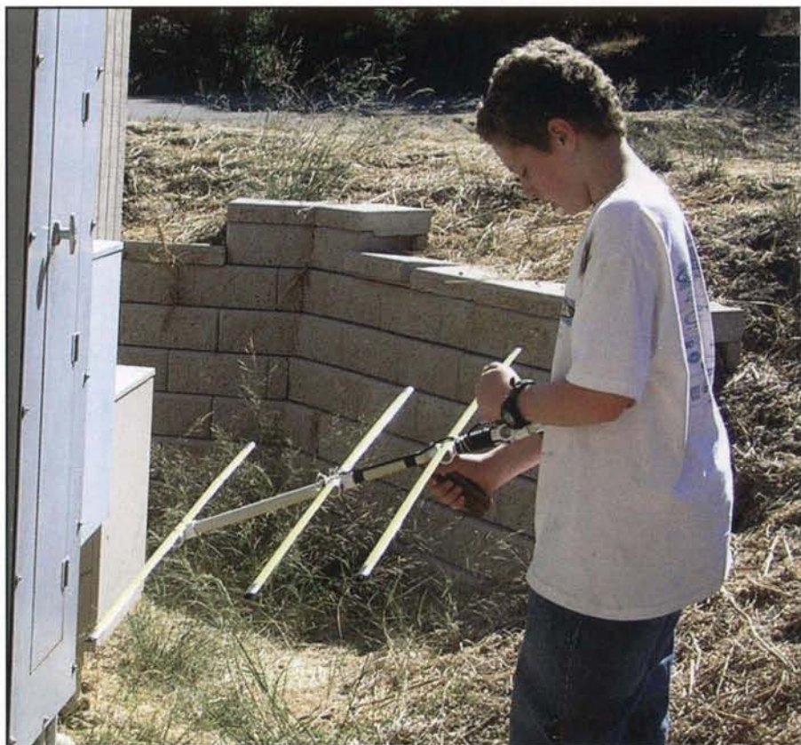
During a Jamboree-On-The-Air event near Santa Barbara, this Scout found it easy to carry my 2-meter measuring-tape Yagi and receiver with one hand using its wooden handle at the balance point. Notice the turns of coax around the boom behind the reflector that serve as a balun. As he closes in on the mini-transmitter, which is behind the conduit below the electrical box, the Scout is using his other hand to shield the receiver from the sun so he can see the display. (Photo by KØOV)
