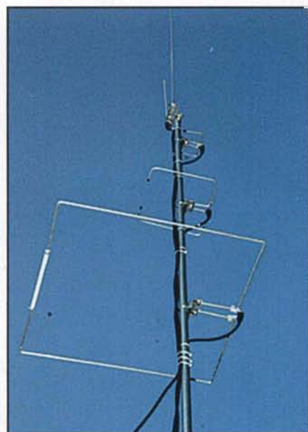
This is a photo of my VHF/UHF stack on the end of the house. In ascending order: KU4AB square Halos for 6 meters, 2 meters, and 70 cm; and a BlueStar 2-meter J-pole on the top for local FM work. Although these antennas are relatively close to the ground (only about 20 feet up), they will be moved to the peak of the roof soon to achieve a total height of about 45 feet. (K7SZ photo)
