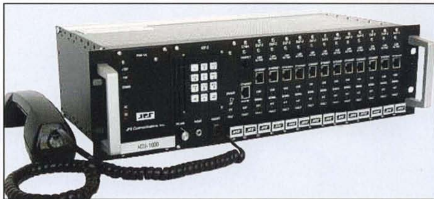
Photo A. Raytheon's ACU-1000 Intelligent Interconnect System.
