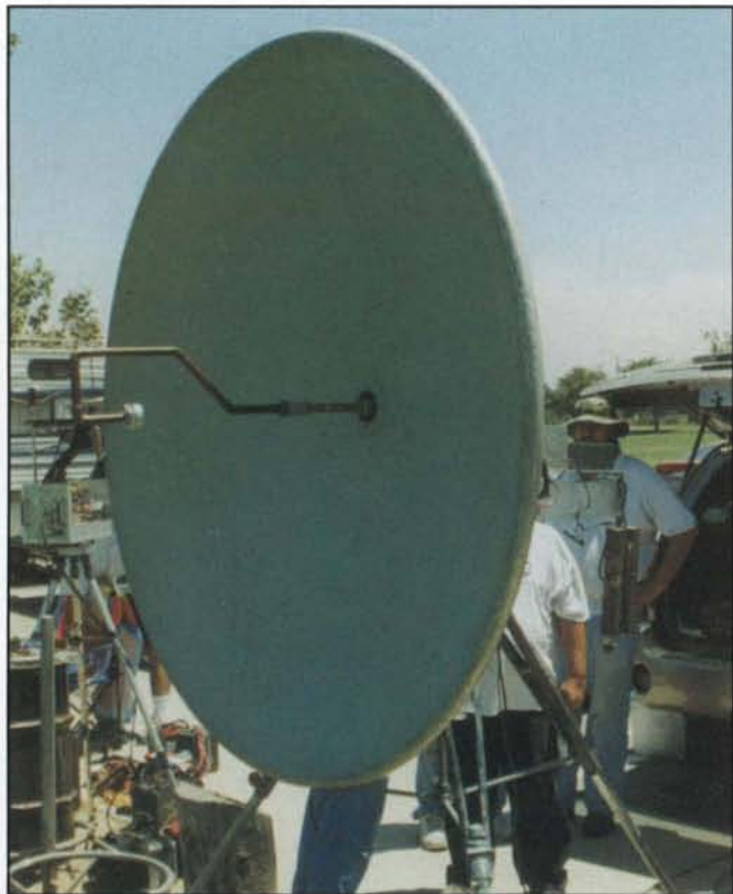
This dish has plenty of gain to work out 700 miles on 10 GHz with 10 watts.
