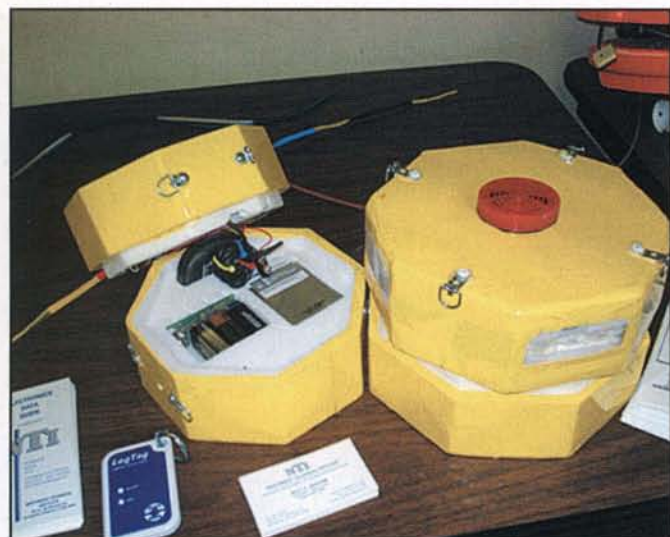
Photo 3. N5NTI payloads with machined Styrofoam for a precision fit.
