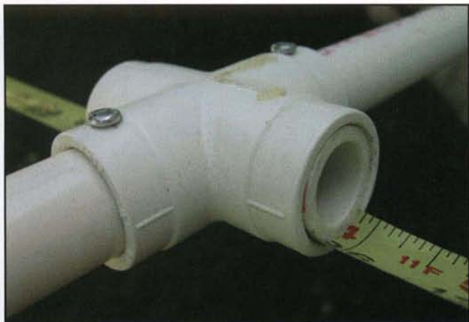
Steve Noskowicz, K9DCI, mounted the elements of his measuring-tape beam inside the PVC couplings, held in place with short lengths of pipe. This eliminated the need for hose clamps or sticky tape. (Photo by K9DCI)
